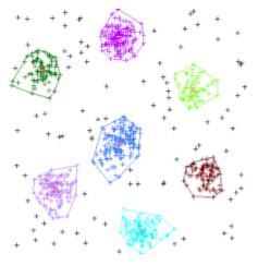
Fig 1. Example of seven clusters determined with the DBSCAN algorithm (in grey are outliers).
