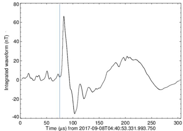
**Figure B** –Magnetic field signal generated by a return stroke located at 46 km from BLESKA. The blue vertical line shows the Météorage’s stroke timestamp corrected for the propagation delay.
