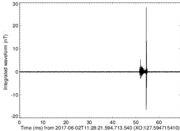
**Figure A** – Part of the long duration record showing the magnetic field waveform related to the preliminary breakdown, the stepped-leader and the return stroke recorded by BLESKA.
