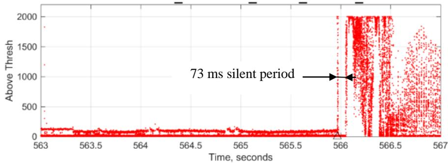
**Figure 1 - Raw data from a SAETTA station that is just below the lightning flash.
