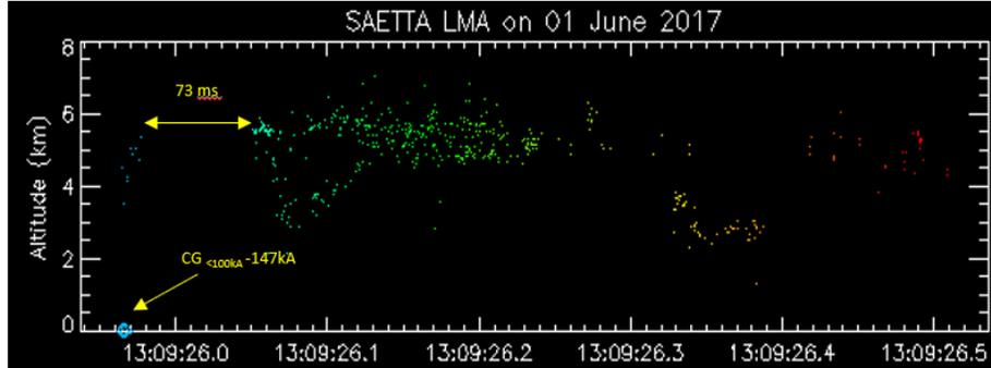
**Figure 2 – Example of a  $-CG_{<100kA}$  flash exhibiting a return stroke of  $-147$  kA observed by both Météorage (blue diamond on X axis) and SAETTA (altitude vs time). One can note the weak VHF activity prior and the silent period (73 ms) after the return stroke.**
